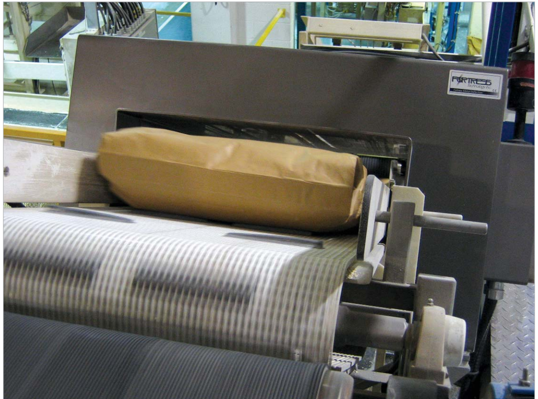
A 50-pound, heavy-duty, heat-sealed, multiwall paperboard filled with oats moves quickly along a Fortress conveyor through a Phantom Big Bag King metal detector at the Can-Oat Milling plant.
